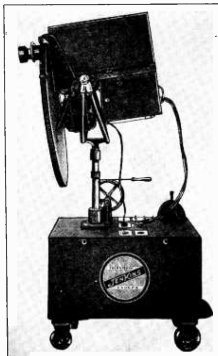
Fig. 5—Latest Jenkins pick-up "camera" suitable for "outdoor" work. It employs a new specially sensitive photo-electric cell.
